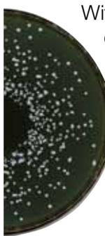
With the **Spiral<sup>®</sup>** method, a **logarithmically decreasing** volume of sample is dispensed on the surface of a rotating Petri dish in an **Archimedes spiral**. The volume is calibrated and known at every point of the Petri dish. Bacterial concentration is determined by dividing the number of colonies found by the volume dispensed in the same sector of the dish.
