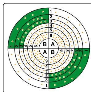
For manual counting, count the colonies in the first A or B outer segment and **reach a minimum of 20 colonies**. Repeat the same operation on the opposite side of the Petri dish.
