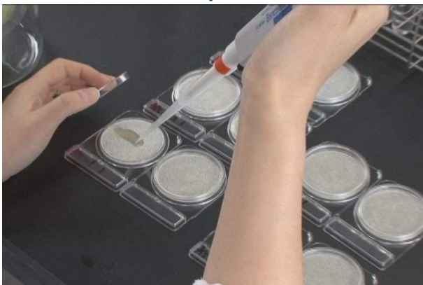
Inoculate the 1 ml sample to the middle of a dry sheet.
